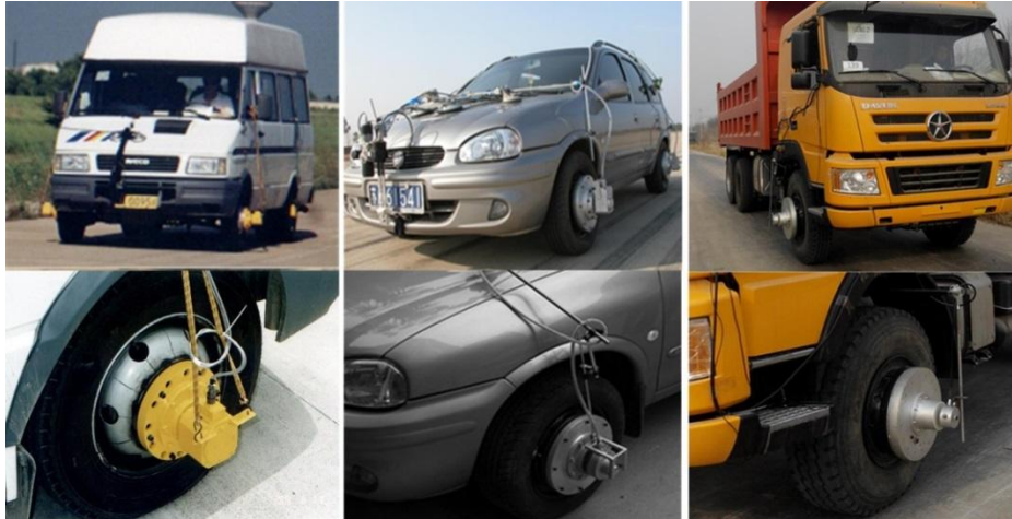
Figure 1. The WFTs developed at SEU (The heavy truck WFT consists the overload protection mechanism in this paper).
